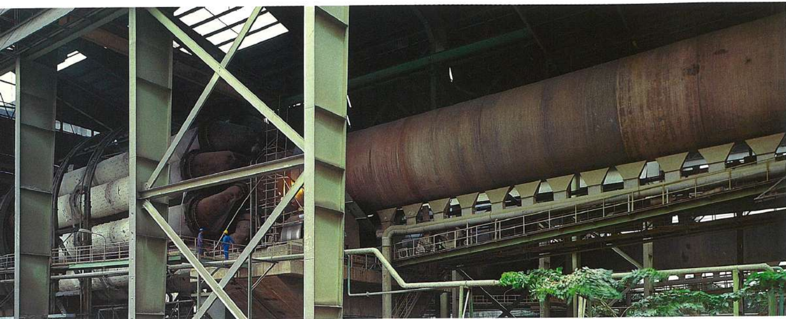
Above: The kiln is used to process the ground raw material to become clinker, an intermediate cement product.
