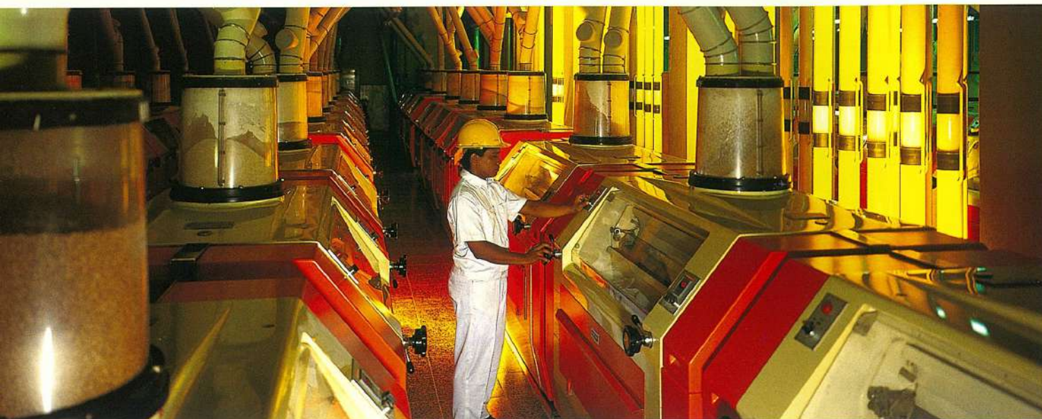
Roller Mills: Wheat is ground and sifted into flour
